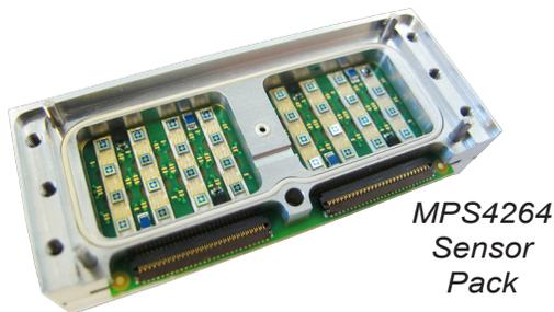
Along with the pressure sensors, all components in the measurement circuit are effected by temperature and drift over time. Scanivalve designed a patent-pending architecture which continuously corrects for these changes over time, while the unit is scanning. This technique of "Dynamic Zero Correction" greatly improves the stability of the entire system over time and temperature. This is accomplished completely "behind the scenes," does not affect performance and requires nothing of the user.
