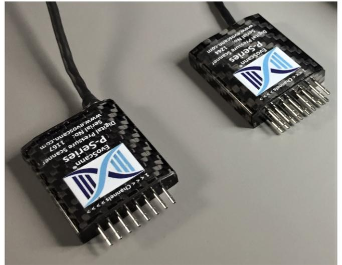
EvoScann® P-Series are highly-miniaturised pressure scanners designed specifically to meet the stringent demands of the aerodynamic testing industry where development is rapid and continuous. Utilising the latest in miniature scanner technology, P-Series is at the forefront of pressure measurement in challenging aerodynamic locations. The P-Series has been designed, from the start, with physical size, weight, accuracy and functionality in-mind and is available in a variety of configurations.
