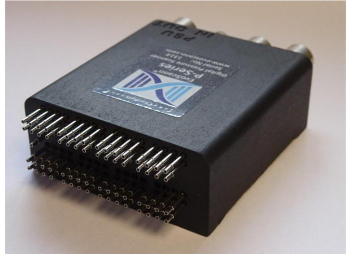
EvoScann® P64-D is a miniaturised pressure scanner designed specifically to meet the stringent demands of the aerodynamic testing industry where development is rapid and continuous. Utilising the latest in miniature scanner technology, P64-D is at the forefront of pressure measurement in challenging aerodynamic locations. The P64-D has been designed, from the start, with physical size, weight, accuracy and functionality in-mind.
