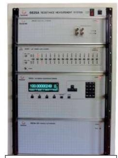
6625-300 Ampere System, from 1 u $\Omega$  to 1G $\Omega$  with single 6664C Scanner
